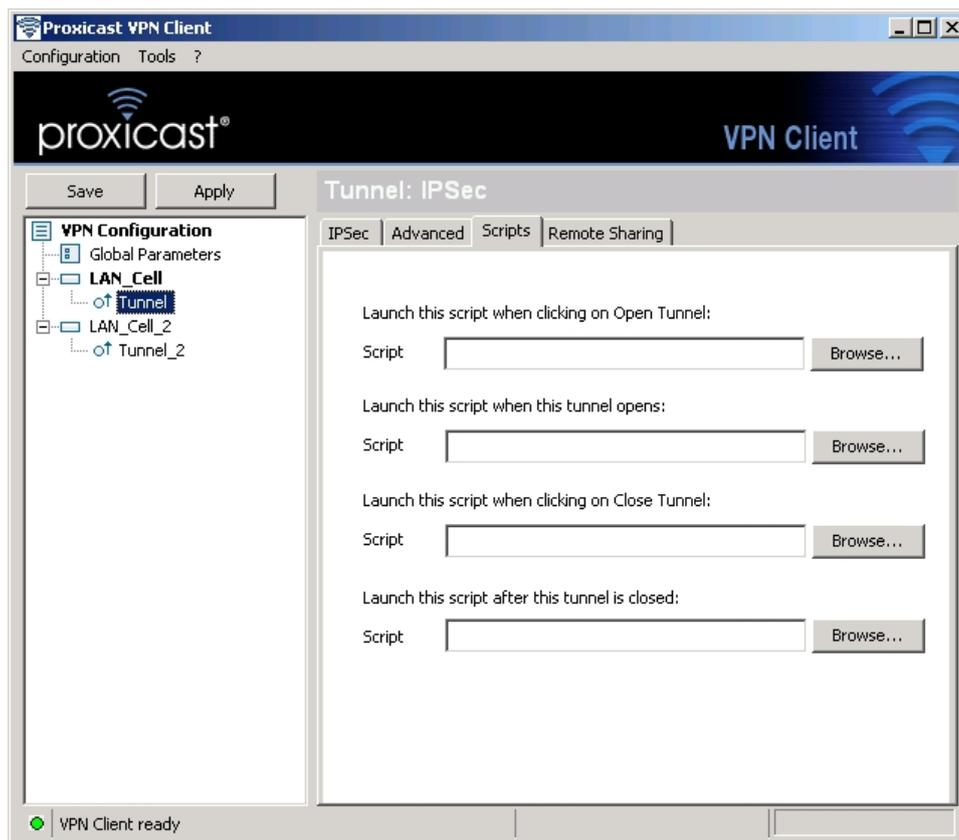
Scripts or applications can be enabled for each step of a VPN tunnel opening and closing process:
