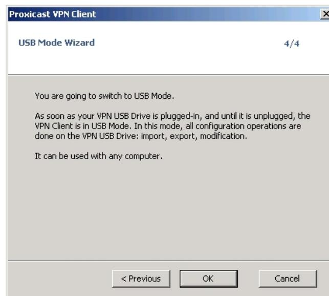
When the USB stick is removed, all configuration information in the VPN Client will be erased. When the USB stick is reinserted, the configuration will be automatically loaded and the USB stick icon will be displayed Configuration and Connection Panels
